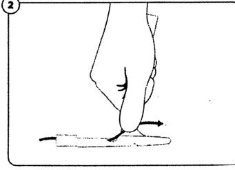
Grip the handle and secure wire(s) with thumb.
