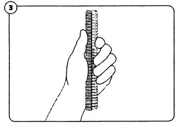
Lightly grip split plastic tubing with opposite hand with the slit facing outwards.
