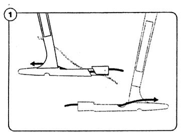
Place wire(s) through the side opening of the Feed Master tool and pivot so that wire(s) are running through the tool and past the handle.
