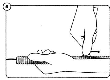
Hold the tube in a stationary position and pull Feed Master through split tube with the other hand while keeping wire(s) in place with thumb.
